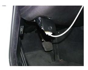
Although it is not required, once you have located your OBD-II connector you might want to note which pin positions are populated (you can usually look into the face of the connector and see which pin positions contain metal contacts). This can be useful in determining what OBD-II protocols your vehicle supports and is extremely helpful if you need to contact us with a connectivity or compatibility problem. Looking into the face of the connector the OBD-II pins are numbered as follows:
