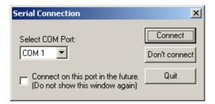
From the drop list, select the COM port assigned to your OT-1 and press the Connect button. Within a few moments, the main, real time display should appear. By default, the first six channels will appear as round gauges. This can be reconfigured (see the <a href="LogWorks User">LogWorks User</a> Manual):
