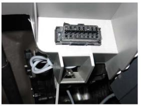
Here is a sample OBD-II connector. Please note that the orientation of the connector varies from vehicle to vehicle.
